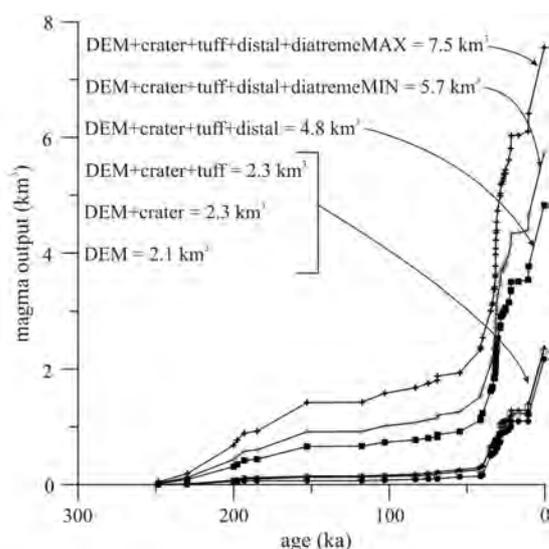
Fig. 2 – The changes of volume output measured. Note: DEM – purely the measurable volume from DEM, crater – magmatic crater infill volume, tuff – volume of circle-based reconstructed tuff ring, distal – volume of distal tephra blanket based minus present tuff ring or scoria cone volume, diatreme MIN and MAX – volumes preserved in the conical and a cylinder-shaped diatreme.
