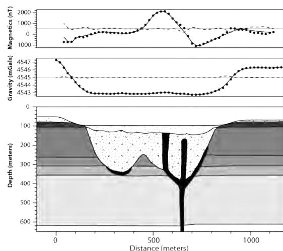
Fig. 2 – 2D forward model of a maar within the RRVC showing two coalesced diatremes and several feeder dykes (Blaikie et al. in preparation).
