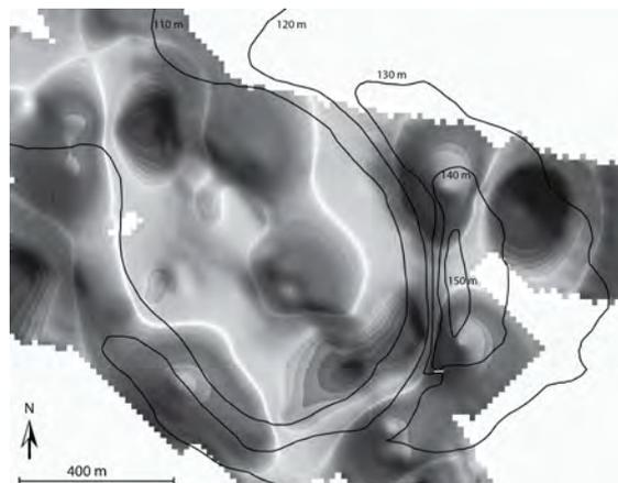
Fig. 1 – High Pass filter (800m cutoff wavelength) of the Bouguer gravity data over Ecklin maar applied to remove a strong regional gradient. Two weak gravity highs can be observed in the centre of the maar and correlate with two magnetic anomalies.
