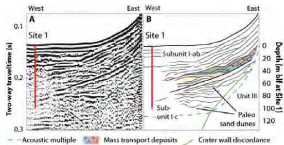
Fig. 3 – Seismic data showing stacked sand dunes overlain by paleo-shorelines (Gebhardt et al., in press).
