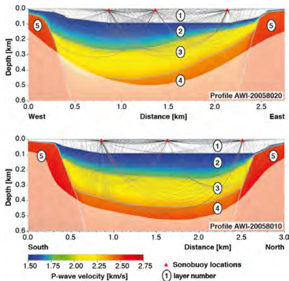
Fig. 2 – Five-layer seismic velocity model of the Laguna Potrok Aike maar (Gebhardt et al., 2011).
