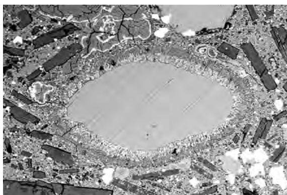
Fig. 3 – Backscattered SEM image showing a reaction rim around a phlogopite crystal. Dark, lath-shaped melilite crystals stand out from a finer matrix. Width of image is 540  $\mu$ m.
