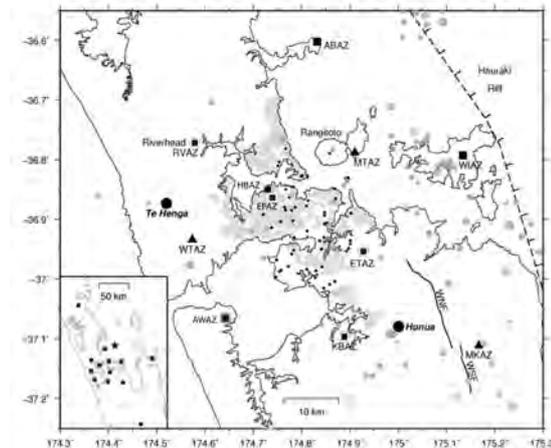
Figure 3. Map of the Auckland region. GeoNet monitors 5 surface seismometers (*black triangles and black squares*) and 6 borehole seismometers (*black rimmed squares*). Earthquakes that occurred between 1980 and 2009 are *grey circles*. Volcanic cones are *small black dots*. Inset shows regional seismic stations (*dots*) and the locations of an earthquake swarm in 2007 (*star*). Modified from Ashenden et al. (2011).
