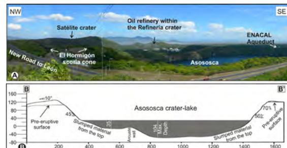
Fig. 2 - A. The Asososca Maar and volcanic structures nearby. The oil refinery of Managua is located inside one of the craters and the ENACAL aqueduct is located on the eastern Asososca crater rim. Scoria cone morphologies (e.g. El Hormigón) are modified by construction and quarrying activities. B. Profile where the morphometric parameters of the Asososca maar can be observed.
