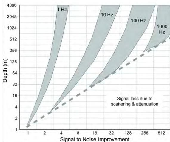
Fig. 2 - Expected improvement of signal to noise ratio with increased seismometer depth. Based on empirical data, Peter Malin and Ashenden et al. (2011).
