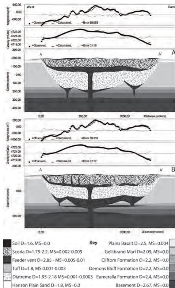
Fig. 1 - 2D forward models across the MNVC, constructed to correspond to east – west magnetic and gravity transects (transect A – A'). Model A displays ponding of rewelded spatter in the crater of the coalesced maars. Model B displays intrusion and inflation of magma along the base of the diatremes.
